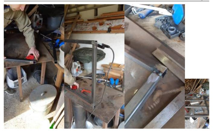
As we decided to use only 2 motors for the first version, we had to improvise a fix for the hoverboard motors. There is a height difference of 9cm between the front wheels and the hoverboard wheels. To have an aligned surface later on, we welded 3 spare pieces together to fix the hoverboard motors onto the chassis.
