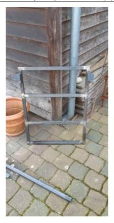
To be able to mount the front wheels and the hoverboard motors onto the chassis, we are using M8 screws. So we drill all the necessary holes into our chassis.
