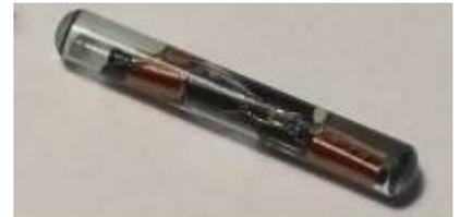
We will document the implanting of the chips we will be getting. We have decided for the [X2.1 Dual](#) implant as our first implant. It includes an RFID 125kHz chip as well as an NFC NTAG216 (13.56MHz) chip in one capsule. The implant measures 15mm in length and 2mm in diameter. It is bigger than the usual 12mm for these kind of implants so it is about the size of 2 rice corns in length.
